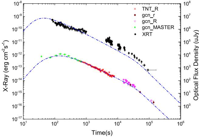
**Figure 4.** Modeling of the optical and X-ray afterglow light curves with the synchrotron external shock model (blue dashed lines). The derived best micro-physical parameters are:  $\Gamma_0 = 315_{-34}^{+44}$ ,  $\epsilon_e = (1.2 \pm 0.1) \times 10^{-2}$ ,  $\epsilon_B = (1.0 \pm 0.1) \times 10^{-6}$ ,  $n = 60 \pm 9 \text{ cm}^{-3}$ ,  $E_{K,\text{iso}} = (1.8 \pm 0.1) \times 10^{55} \text{ erg}$ ,  $p = 2.72 \pm 0.07$ , and  $\theta_j = 0.04_{-0.01}^{+0.02} \text{ rad}$ .
