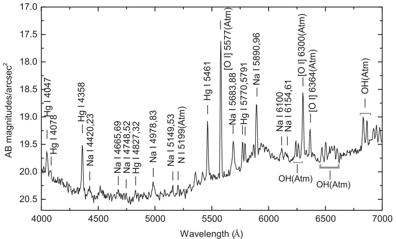
**Figure 2.** A typical spectrum in the range of 4000 to 7000 Å of the night sky at Xinglong Observatory. Emission lines from natural (atmosphere) and artificial (Hg and Na) sources are identified and marked.
