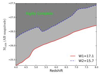
**Figure 1.**  $M_{1450}$  as a function of redshift for a type I quasar template from Glikman et al. (2006). The red solid line denotes W1 = 17.1 and the blue dashed line denotes W2 = 15.7, which are the 95% completeness limits of the ALLWISE catalog. ALLWISE is a promising data set for finding high-redshift quasars with high luminosity (e.g.,  $M_{1450} \leq -26.5$  at  $z \leq 6$  and  $M_{1450} \leq -27.0$  at  $z \leq 7$ ).
